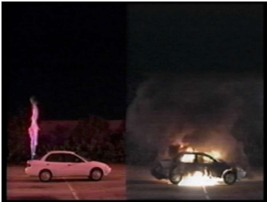
Figure 5 - Simulation Time: 1 min, 0 sec - Hydrogen flow is subsiding, view of gasoline vehicle begins to enlarge. (Fuel Leak Simulation Dr. Michael R. Swain)
