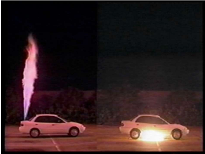
Figure 4 - Simulation time: 0 min, 3 sec – Ignition begins, Hydrogen powered vehicle on the left. Gasoline powered vehicle on the right. (Fuel Leak Simulation Dr. Michael R. Swain)
